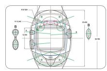
Graphite 2D/3D CAD software is used to determine the best layout for the watch components and communicate with manufacturing in 2D drawings.
